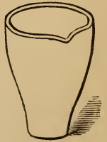
London clay crucible for refining gold.
